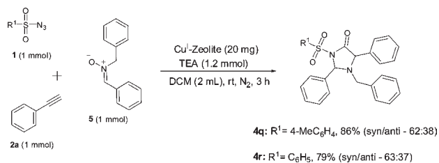
Scheme 2. Copper(I)-Catalyzed Cascade Synthesis of Imidazolidin-4-ones from N -Benzylnitrones
